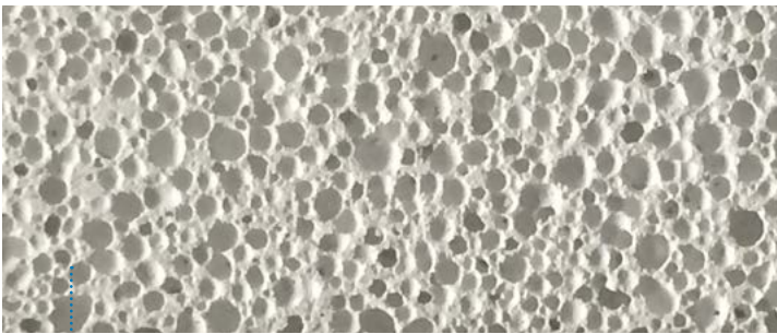
Fig. 1: Example of pore structure of AAC (Yitong, Changxin)
